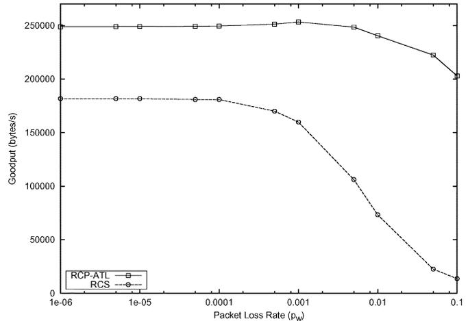
Fig. 14. Goodput comparison of RCP-ATL and RCS for  $d_w = 150$  ms and varying  $p_w$ .
