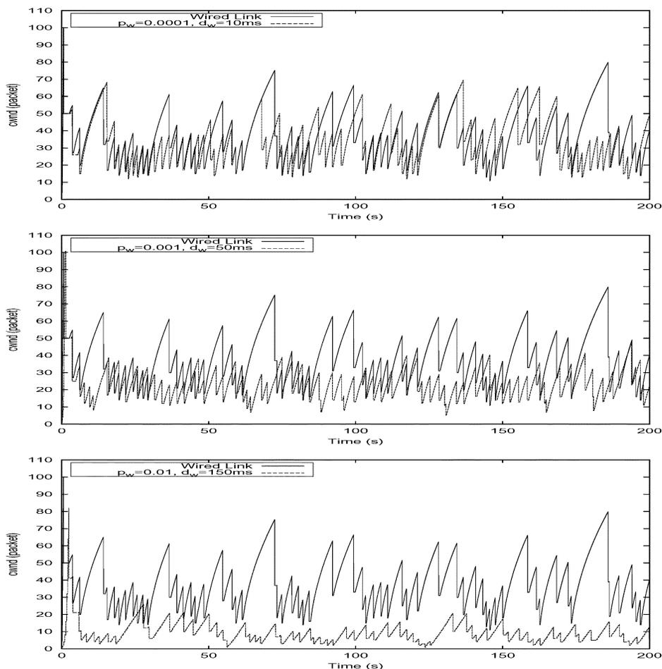
Fig. 2. Congestion window change with time for different wireless link conditions.
