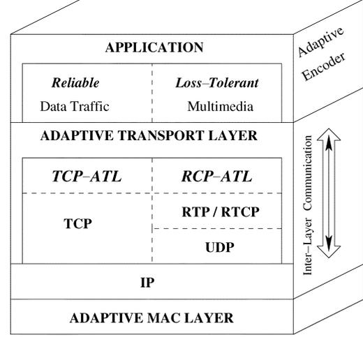
Fig. 3. Typical protocol stack including ATL.
