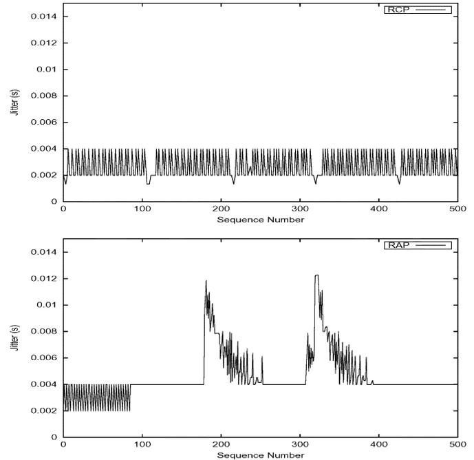
Fig. 17. Jitter experienced by the RCP-ATL and RAP packets for  $d_w = 10$  ms and  $p_w = 10^{-4}$ .
