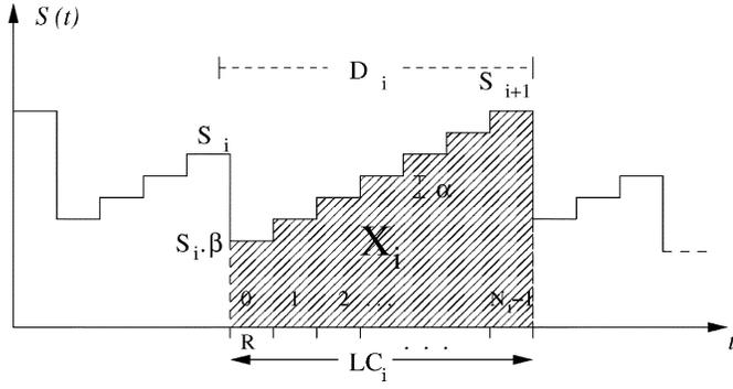
Fig. 18. Data rate change of rate-base general AIMD congestion control.
