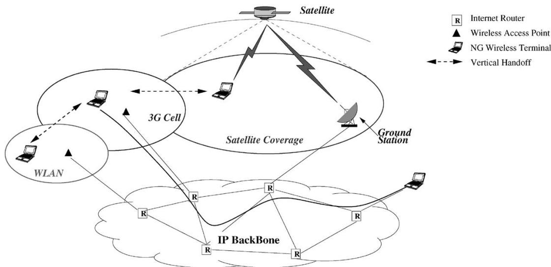
Fig. 1. Typical proposed NGWI architecture including WLAN, 3G, and satellite networks converged with the next-generation Internet backbone.
