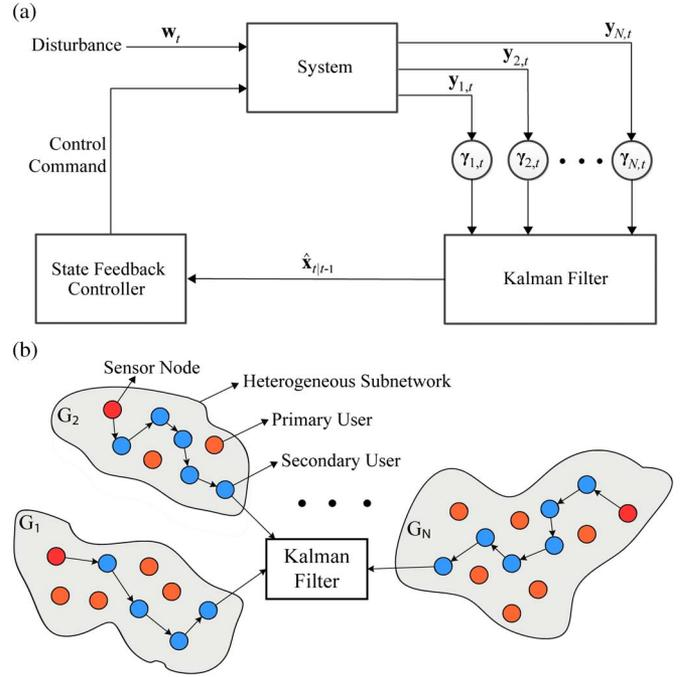
Fig. 1. (a) Block diagram of the WNCS. (b) Model of the heterogeneous multi-hop wireless *ad-hoc* subnetworks.
