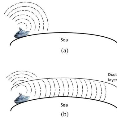
Fig. 1. Signal spreading in (a) standard atmosphere and (b) duct.
