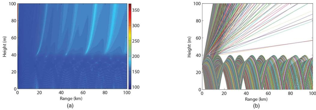
Fig. 3. Wave propagation results with (a) PETOOL and (b) RO methods for 40-m surface duct, 10 GHz, 27-m transmitter height.
