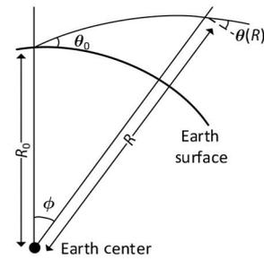
Fig. 13. Ray trajectory for refractive path.
