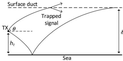
Fig. 14. Trajectory of a trapped ray.
