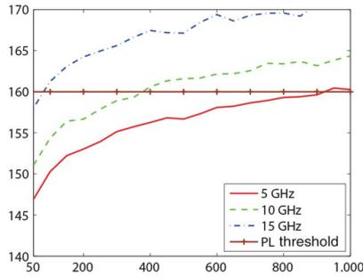
Fig. 12. Link budget analysis for surface ducts.
