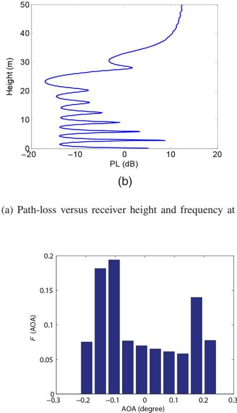
Fig. 10. Histogram of AOA for a 40-m surface duct.
