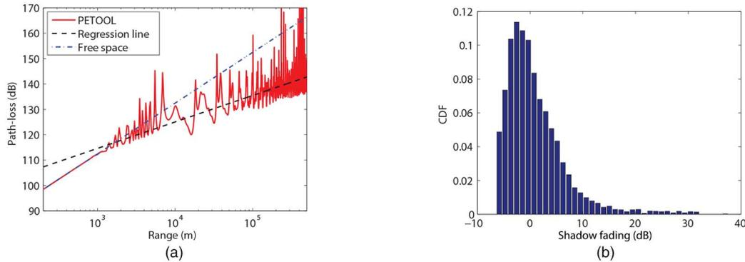
Fig. 5. Path-loss results for (a) regression method and (b) distribution of the shadow fading.
