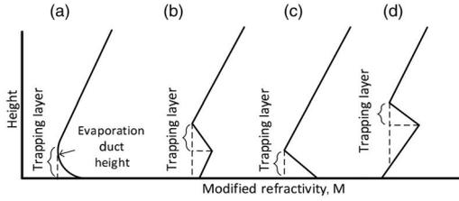
Fig. 2. Modified refractivity profiles of atmospheric ducts. (a) Evaporation duct. (b) Surface-based duct. (c) Surface duct. (d) Elevated duct.
