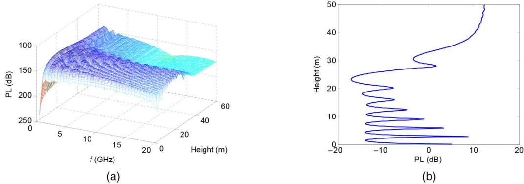
Fig. 8. Path-loss results for 40-m surface duct, 27-m transmitter height with PETOOL. (a) Path-loss versus receiver height and frequency at 100-km range. (b) Receiver height versus path-loss at 100-km range.
