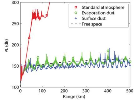
Fig. 7. Path-loss versus range for standard atmosphere, free space, and atmospheric ducts.
