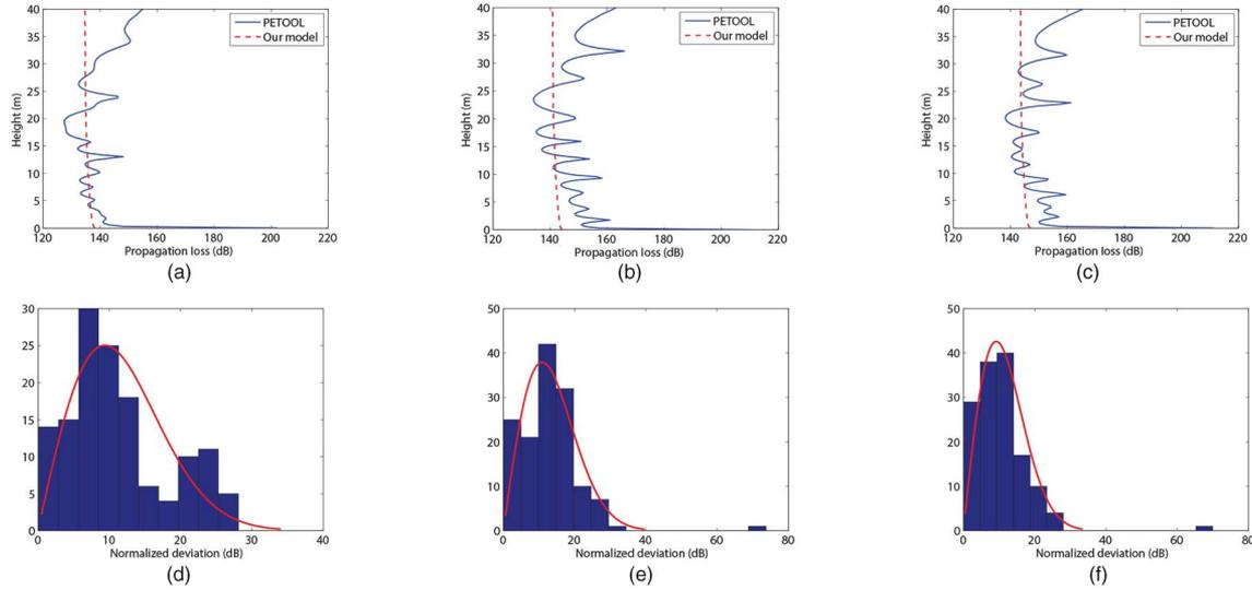
Fig. 11. Comparison of our large-scale path-loss model and PETOOL results. Comparison at (a) 50; (b) 250; and (c) 500 km. Histogram of deviation at (d) 50; (e) 250; and (f) 500 km.
