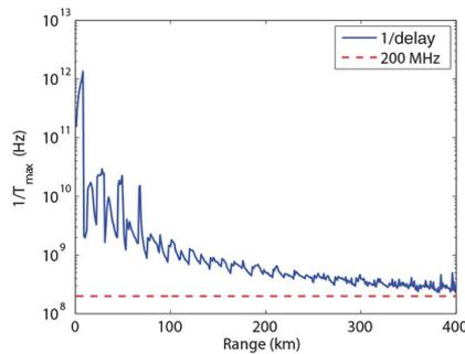
Fig. 9.  $1/T_{max}$  spread for a 40-m surface duct.
