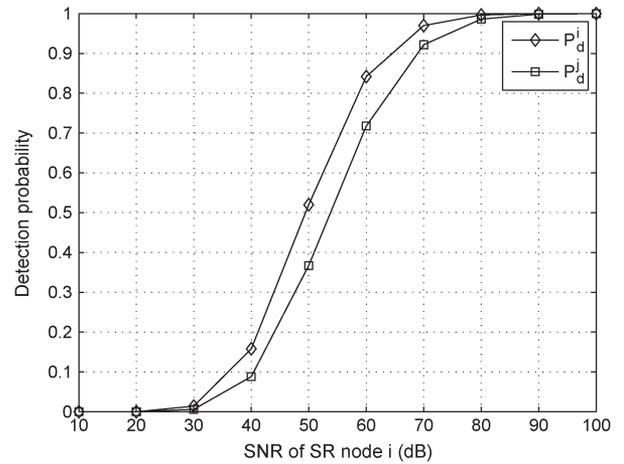
Fig. 2. Detection probability of SR node  $n_i$  and correlated node  $n_j$  for different SNR values  $\gamma_i$ , where  $\theta_d = 10000$ ,  $\lambda = 100$ ,  $\alpha = 2$ , and  $d_{i,j} = 20$  m.
