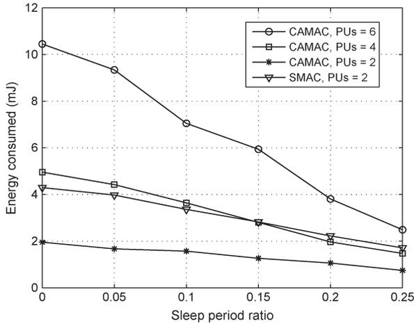
Fig. 7. Average energy consumption per SU at varying sleep period ratio of a duty cycle.
