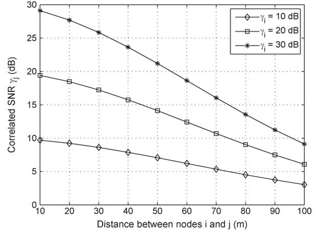
Fig. 1. Correlation of SNR values at different distances between nodes  $n_i$  and  $n_j$ , where  $\theta_d = 10000$ .
