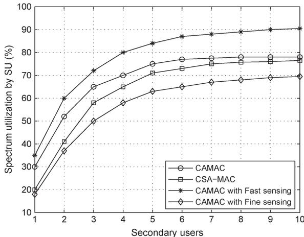
Fig. 5. Spectrum utilization comparison of the proposed CA-MAC with the existing CSA-MAC protocol [4].
