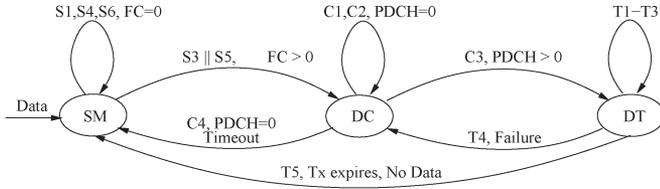
Fig. 3. CAMAC phase transition diagram to illustrate its MAC operations.
