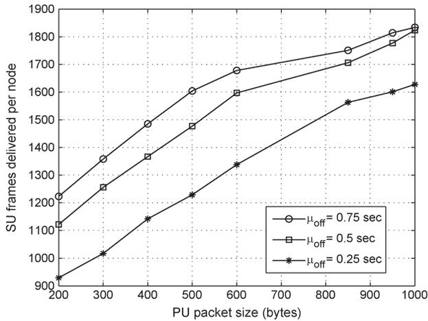
Fig. 10. SU frames per node delivered at different frame sizes of PUs at a fixed traffic rate.
