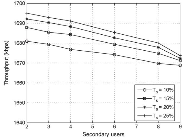
Fig. 9. Throughput of PUs by varying the number of SUs at different values of  $T_s$  ratio.
