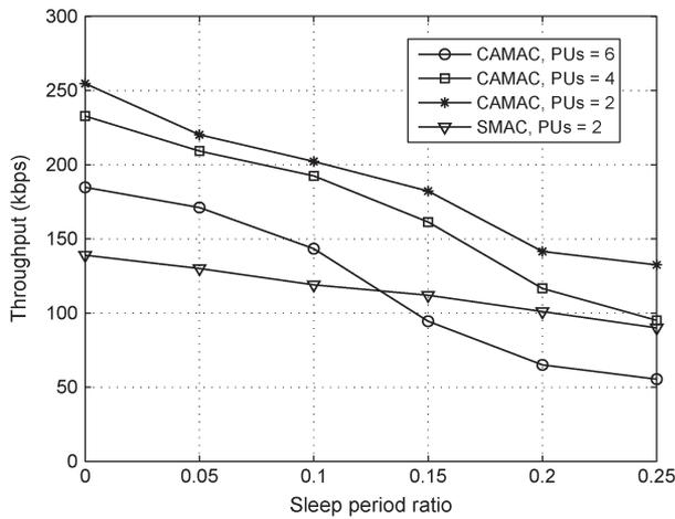
Fig. 8. Average SU throughput at different sleep period ratio of a duty cycle.
