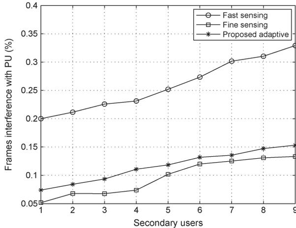
Fig. 4. SU interference with the PUs using different sensing mechanisms.
