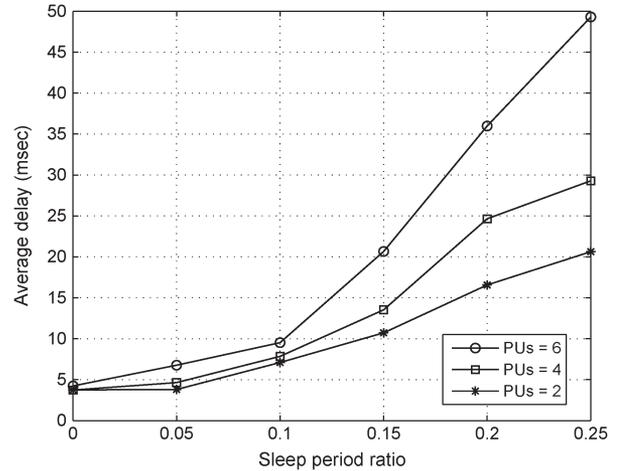
Fig. 6. Average frame delay of SUs at different values of  $T_s$  ratio in a duty cycle.
