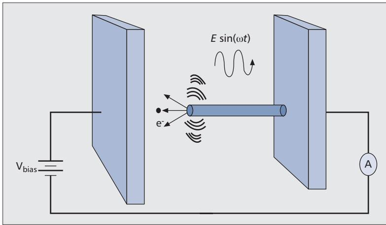
Figure 1. Illustration of nanotube radio circuit [6].
