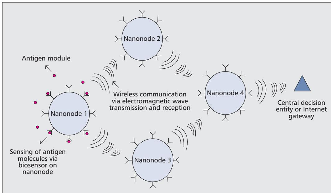
Figure 3. Illustration of a CANET application example, i.e., nanoscale bio-sensor network.
