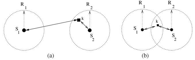
Fig. 2. (a) Source-to-source interference, (b) source-to-node interference.
