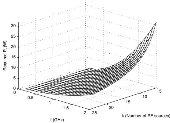
Fig. 4. Required RF power for number of RF sources and frequency.
