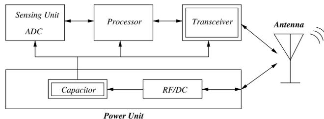
Fig. 1. Building blocks of a typical WPSN node.
