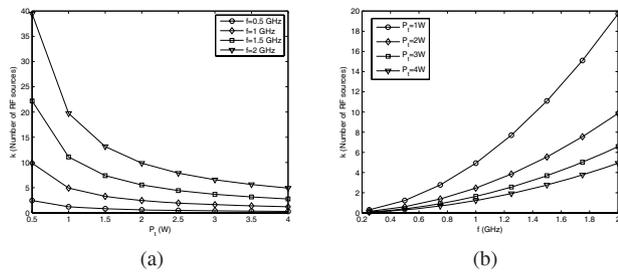
Fig. 3. Variation of  $k$  with (a) RF output power, (b) carrier frequency.
