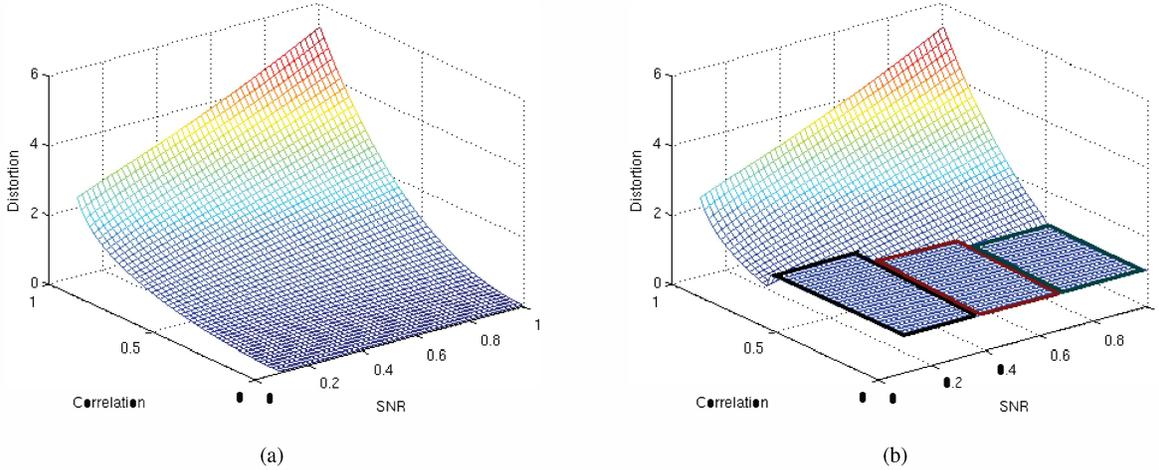
Fig. 1. Distortion in sufficient statistics and corresponding admittance regions
